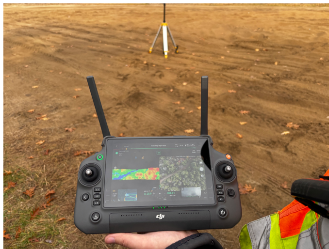
Figure 6. The LiDAR view on a drone controller during the survey. Photo by Susannah Clinker.
